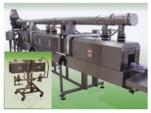
The compact KST80-712 steam tunnel (inset) can be connected to another unit (main image) if line speeds or container size and shape require more time in the tunnel.
